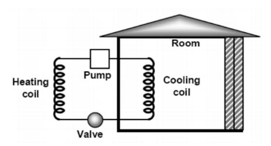
The outside air temperature is  $T_{\rm H}$  and the inside air temperature is  $T_{\rm L}$ . The air conditioner unit consumes electric power P. Assume that the air is dry sufficiently so that no condensation of water occurs in the cooling coils of the air conditioner. Which of the following may be the rate at which heat is removed from the room?
